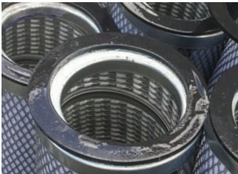
FIGURE 4. Shown here are coalescer elements with flat gaskets that have swelled and extruded out of place due to compatibility issues with the fluids they encountered during operation. Gasket swelling weakens the seal, creating leakage pathways
