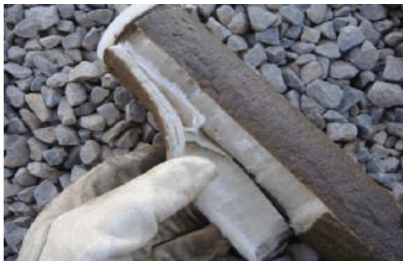
FIGURE 5. Use of a filter element with incorrect media is a common problem. As seen in this example, contaminants accumulated at the surface of the filter element, but were blinding the media, preventing smaller contaminants from reaching the inner tapered-pore media, and resulting in reduced capture efficiency and shortened filter life
