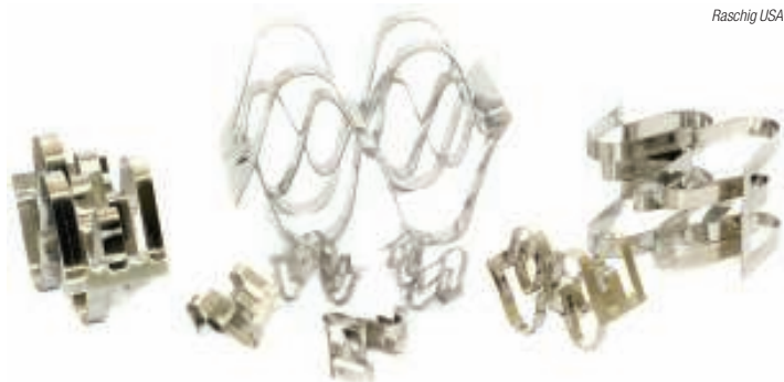
FIGURE 1. The Raschig Super-Ring offers a grid-like structure that provides a lower resistance to gas flow, reduces pressure drop and results in improved capacity compared to earlier packings
