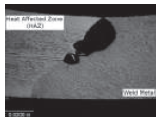
FIGURE 3. This magnified cross section of a weld in a stainless-steel pipe reveals a cave structure that confirms MIC. The cave structures typically occur at the boundary between a weld and the base metal
