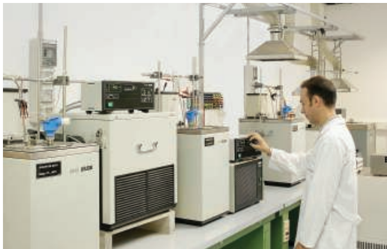
FIGURE 6. Many laboratories can calibrate sensors and transmitters, and determine CVD constants for an RTD and probe
