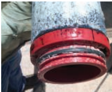
FIGURE 6. Due to the use of an incompatible lubricant grease, the lubricant solidified, cementing the elements into the vessel. The need to use force to remove the filter elements damaged the risers on which the elements sit
