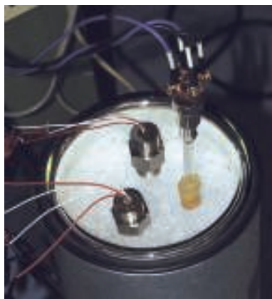
FIGURE 2. RTD probes are immersed in an ice bath at 0°C for testing and classification purposes
